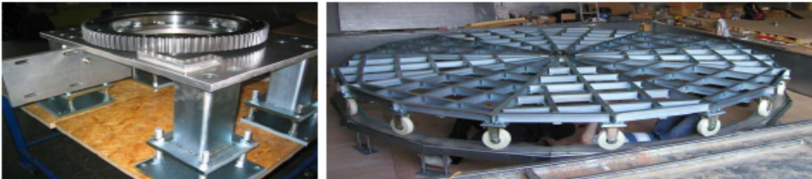
Figure: Level system of turntable for height adjustment
